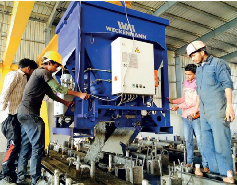
*Important for the dimensional accuracy and surface finish: homogeneous distribution of the concrete.*
