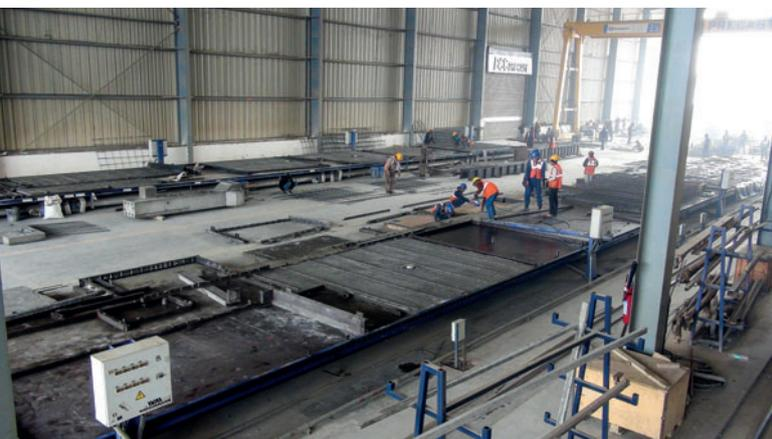
*Production of precast slabs with in-situ topping in the Weckenmann precast plant in Bharat City, India.*
