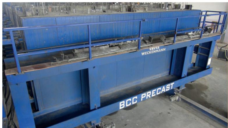
*One of the two battery moulds for the interior and exterior walls.*
