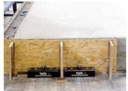
The MagnetBox can also be used to support shuttering
