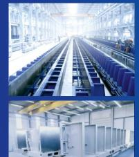
**CASTING BEDS** are perfectly suited to produce prestressed floor slabs economically and efficiently. The consistent design and **individual optimisation of the production lines** are the alpha and omega in this regard. Our support for our customers already starts with the planning stage to ensure efficient processes all the way from concrete supply to loading for transport.
