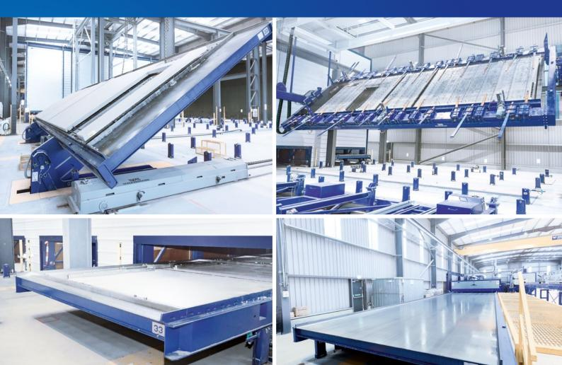
PALLET TRANSPORTATION to transport the pallets within the circulation system, the transportation technology at Weckenmann comprises the complete range of individual handling technologies. Depending on the design of the material flow concept, individual workstations are networked through friction wheels, cross lifting trucks, central transfer tables, central sliding stages or by a combination of these components.
