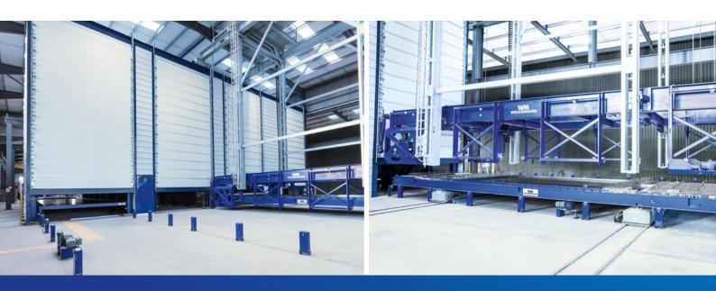
**CURING CHAMBER** for heat-insulated, controlled and space-saving **curing of concrete elements.** If necessary, this process can also be accelerated by built-in air conditioning/heating.
