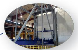
Full automatic **storage and retrieval** crane and curing chamber. Heating by computer controlled hot air ventilation.
