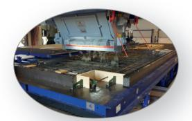
**Concrete spreader** with two swap buckets to process two different concrete recipes at the same time.
