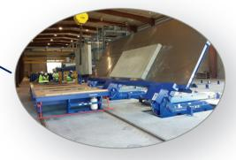
**Tilting station** to bring the pallet to an almost vertical position for shipping wall panels.
