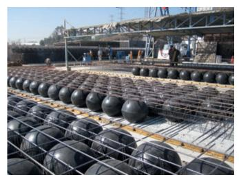
The Mexican company mainly uses the new production facility for the manufacture of biaxial carrying hollow decks, which are also known as Bubble Decks due to their round displacement bodies.
