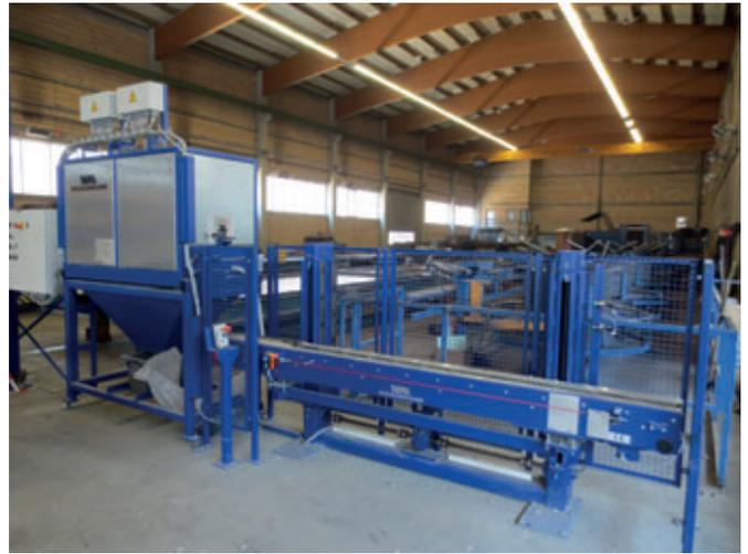
*Afterwards: Shuttering transport with cleaner/oiler for shuttering with integrated magnets. Automatic cleaning/oiling of the shuttering and transport of the shuttering from the demoulding station direct to the shuttering station.*
