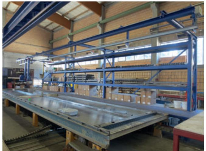
*Afterwards: On the left the new state-of-the-art storage, cleaning and plotting device with new controller. On the right the manual shuttering station in the form of the workplace system with mobile tool trolley, hot-glue gun, manual oiler, rack system and gangway alongside the pallet. Control consoles for pallet movement directly adjacent to the work station. On the pallet is fresh shuttering with integrated magnets.*
