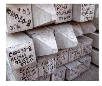
The Weckenmann experts have also designed the new bulkhead for the typical pile tips. With this, flat tips can now be produced for extension piles in addition to the pointed tips. For removal the bulkhead can be opened completely, so that the finished piles can be lifted out vertically. The result is a lower risk of accidents for the employees and no risk of damaging the finished products.
